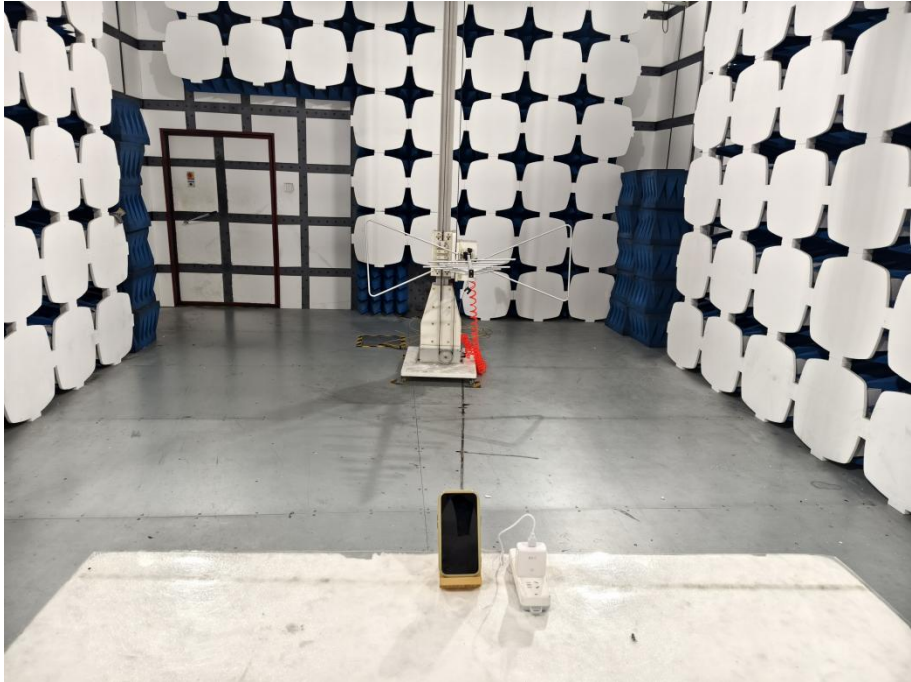
Photo of Radiated Emissions Measurement
