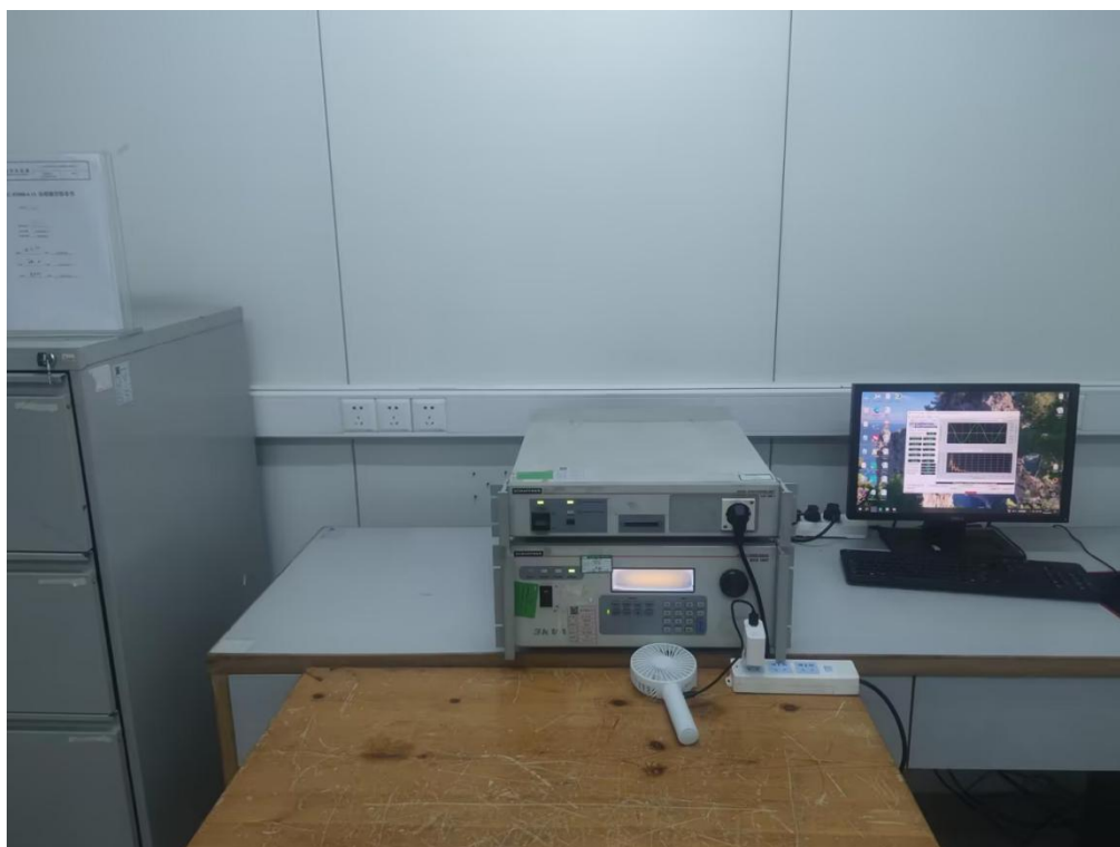
Harmonic current emissions & Voltage fluctuations and flicker
