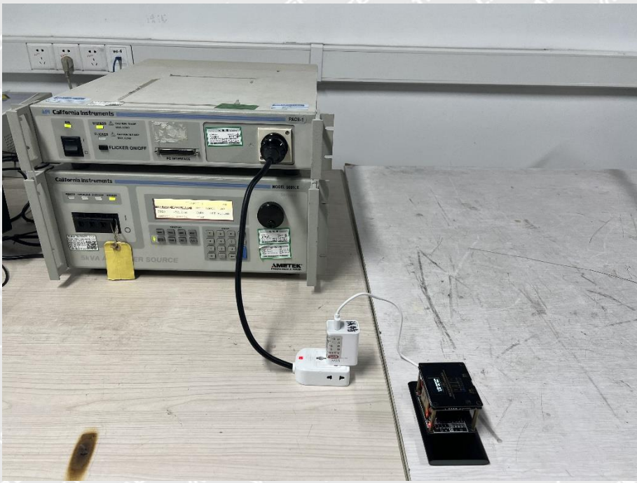
Harmonic/Flicker Test View
