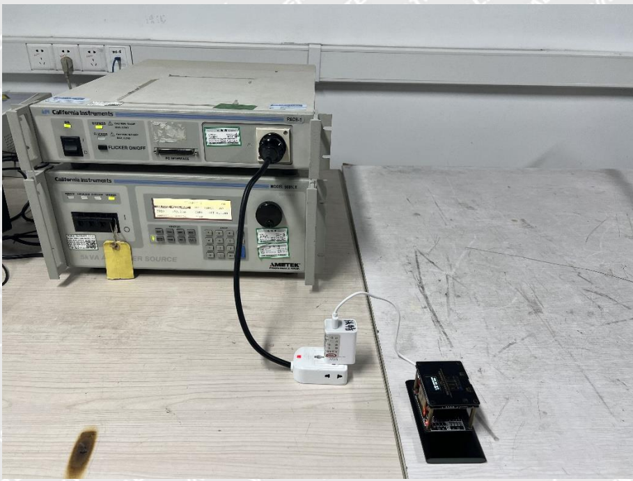
Harmonic/Flicker Test View
