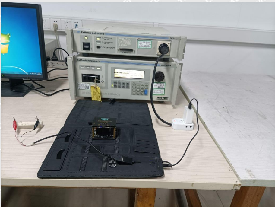
Harmonic/Flicker Test View
