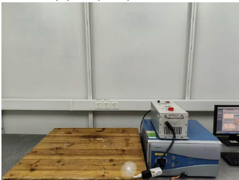
EN 61000-4-4/-5/-11 EFT/SURGE/DIPS IMMUNITY TEST SETUP
