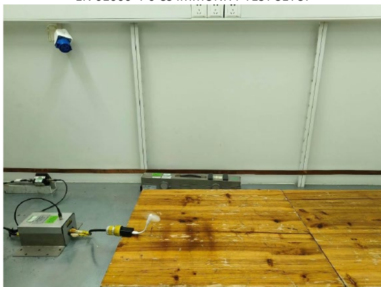
EN 61000-4-6 CS IMMUNITY TEST SETUP
