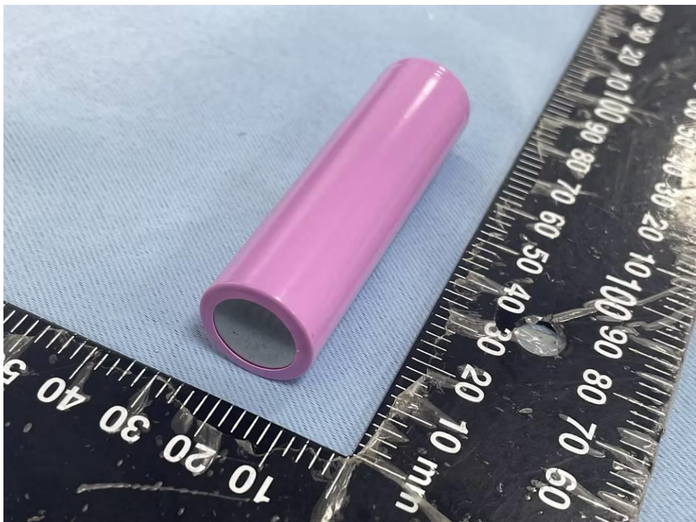
Picture 8 Bottom view of cell (Model: INR18650L22)
