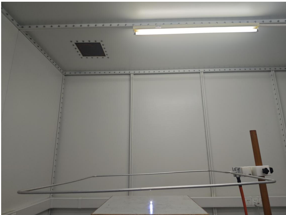
Measurement of Power Frequency Magnetic Field
