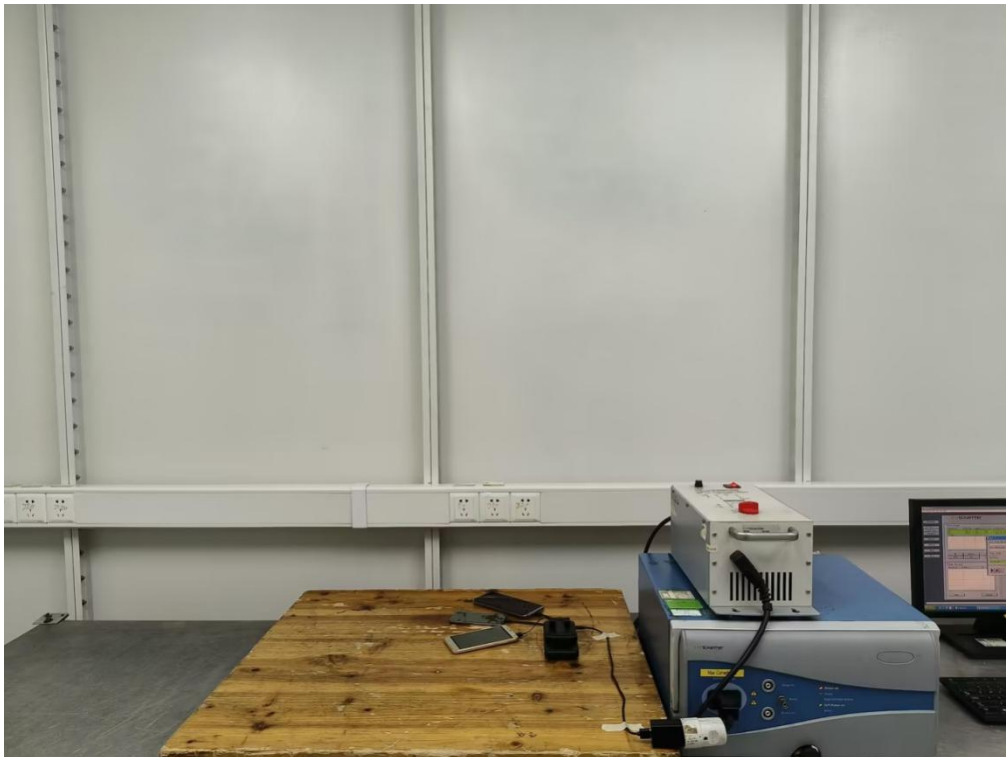
EN 61000-4-4/-5/-11 EFT/SURGE/DIPS IMMUNITY TEST SETUP
