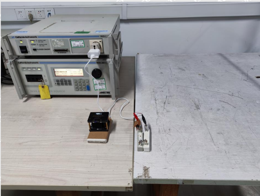
Harmonic/Flicker Test View
