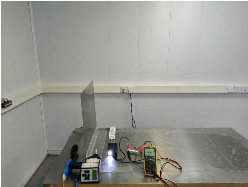
Test Setup Photo of Electrostatic Discharge Test
