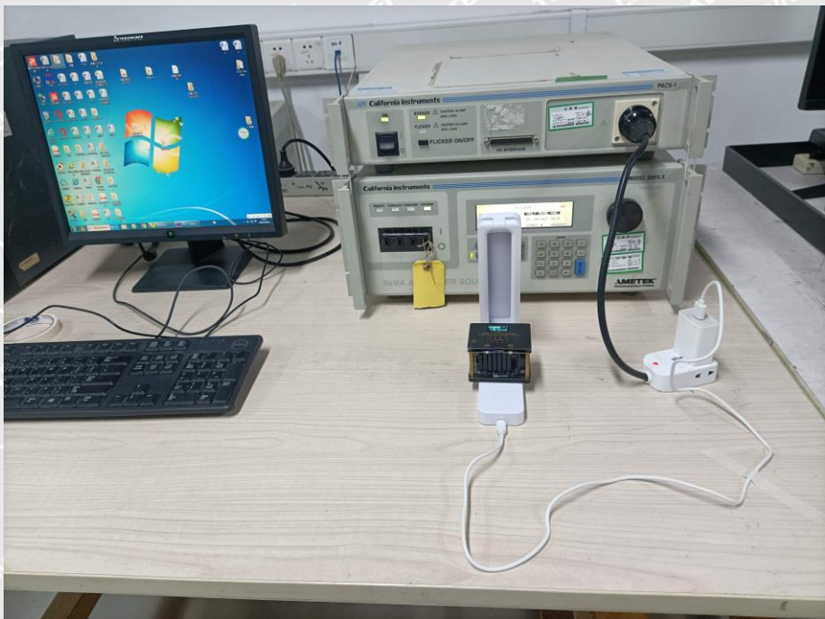
Harmonic/Flicker Test View
