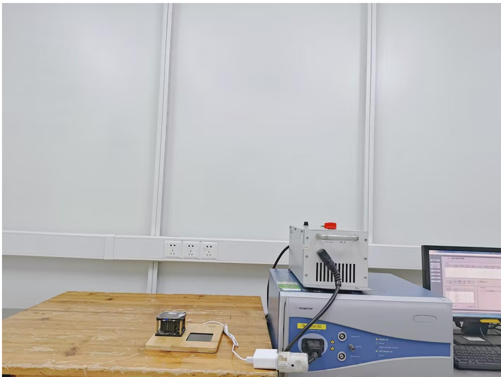
EN 61000-4-4/-5/-11EFT/SURGE/DIPS IMMUNITY TEST SETUP
