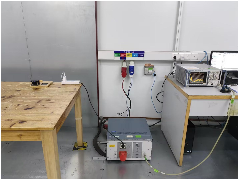
RADIATED EMISSION TEST SETUP (Below 1GHz)
