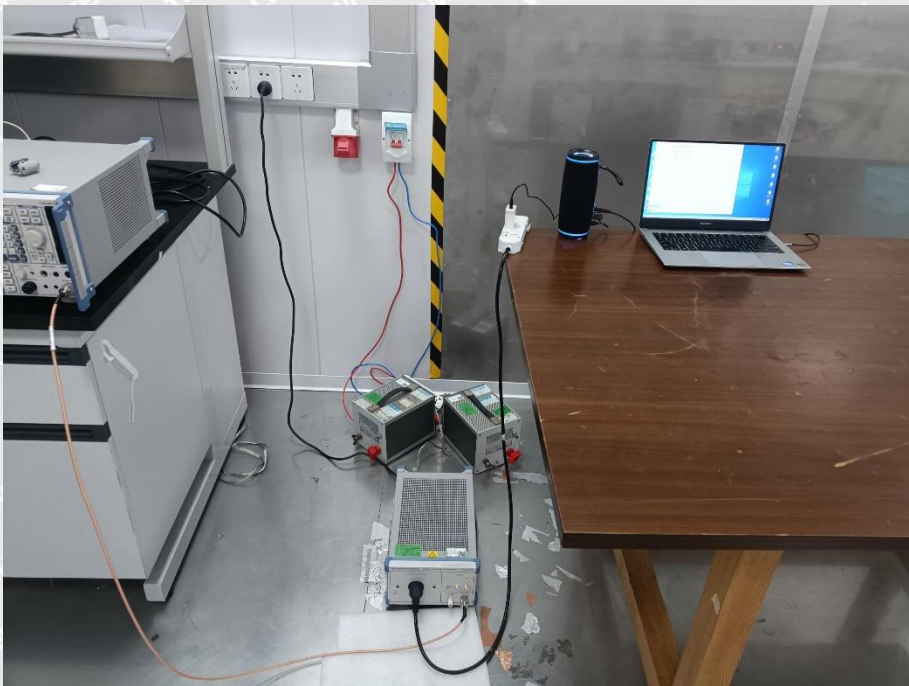
Conducted Emission Test Setup
