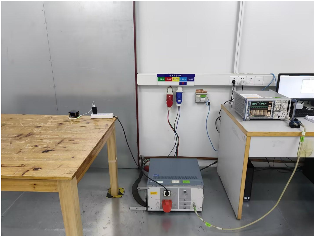
RADIATED EMISSION TEST SETUP (Below 1GHz)
