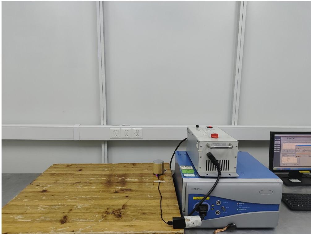
EN 61000-4-4/-5/-11 EFT/SURGE/DIPS IMMUNITY TEST SETUP
