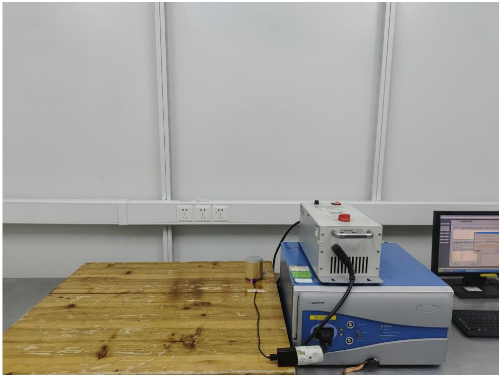
EN 61000-4-4/-5/-11 EFT/SURGE/DIPS IMMUNITY TEST SETUP
