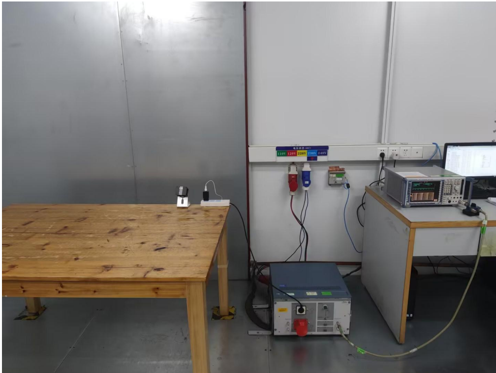
RADIATED EMISSION TEST SETUP (Below 1GHz)
