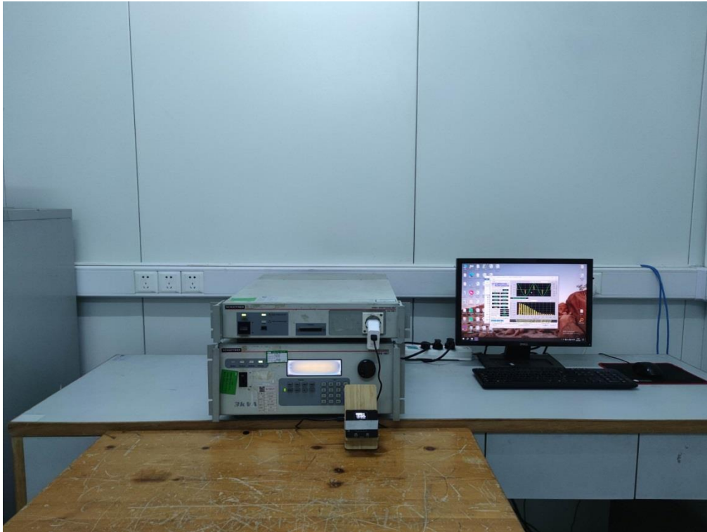
Harmonic Current Emissions & Voltage Fluctuations and Flicker
