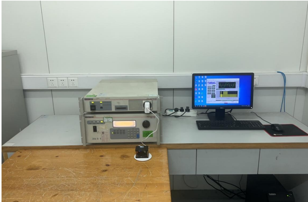
Harmonic Current Emissions & Voltage Fluctuations and Flicker
