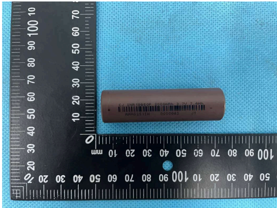
Figure 9 Front view of cell (Model: INR 18650P-2000mAh)
