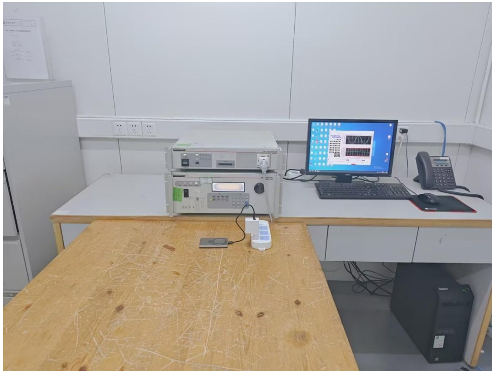
Harmonic current emissions & Voltage fluctuations and flicker
