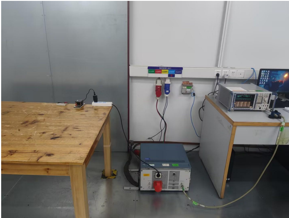
RADIATED EMISSION TEST SETUP (Below 1GHz)
