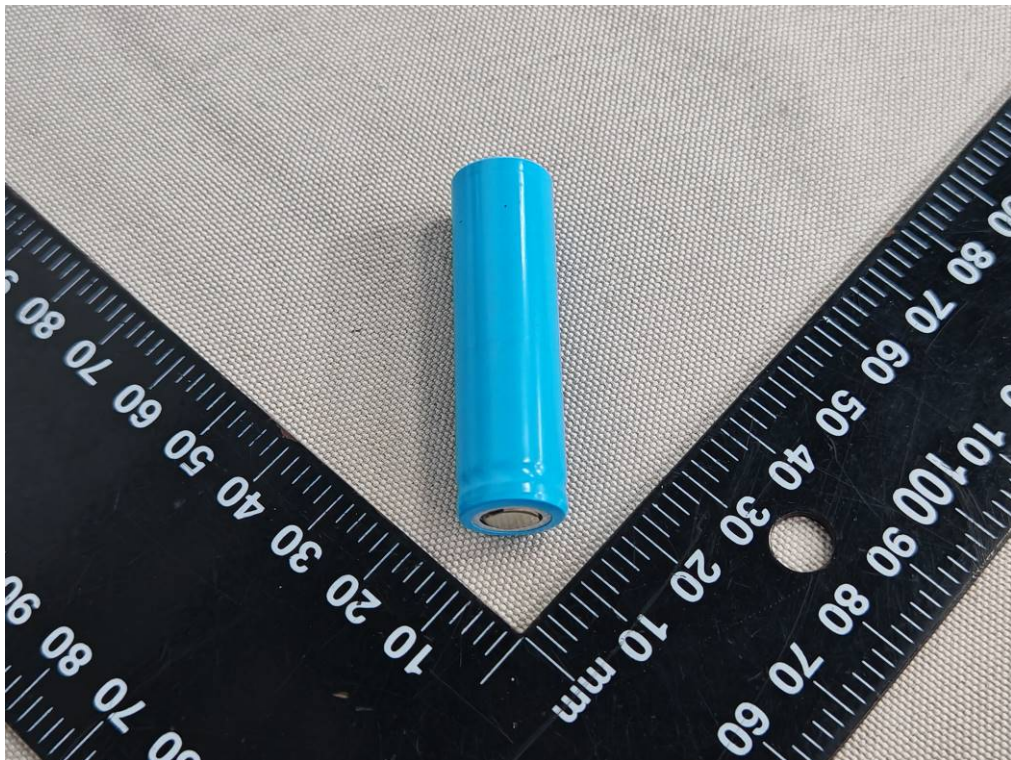
Figure 8 Side view of cell (Model: IMR14500-300mAh)
