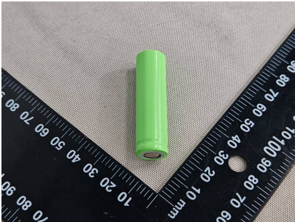
Figure 4 Side view of cell (Model: IMR14500-500mAh)
