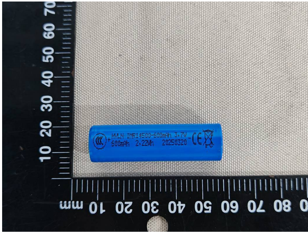
Figure 5 Front view of cell (Model: IMR14500-600mAh)
