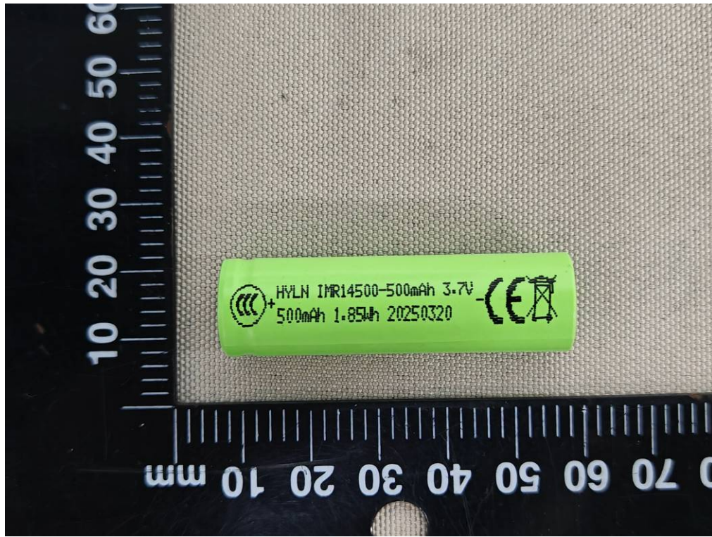
Figure 3 Front view of cell (Model: IMR14500-500mAh)
