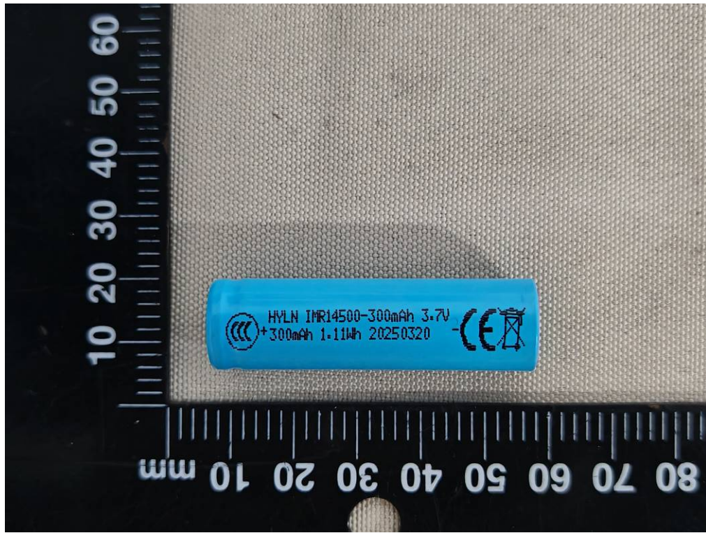
Figure 7 Front view of cell (Model: IMR14500-300mAh)
