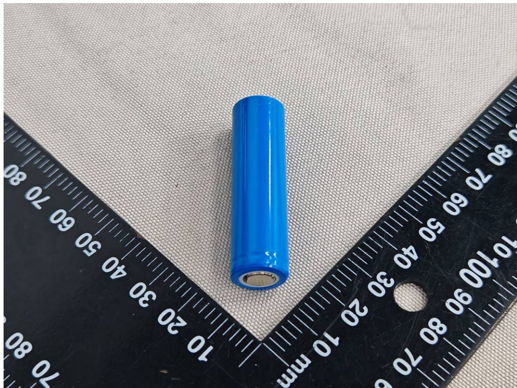
Figure 6 Side view of cell (Model: IMR14500-600mAh)
