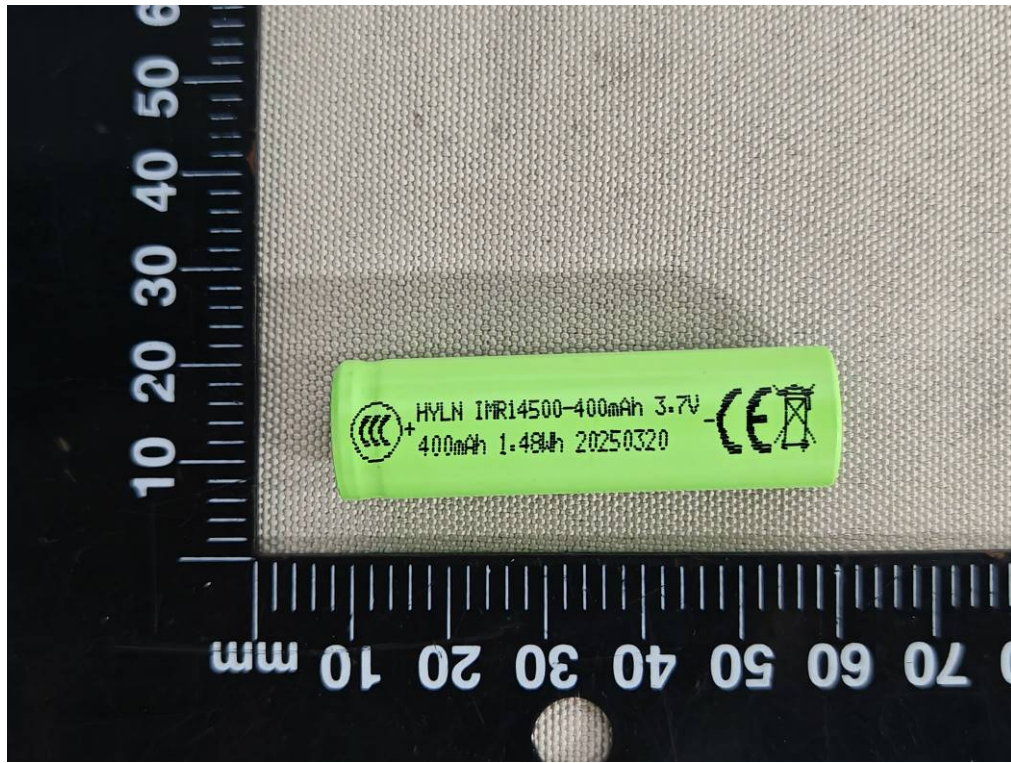
Figure 1 Front view of cell (Model: IMR14500-400mAh)
