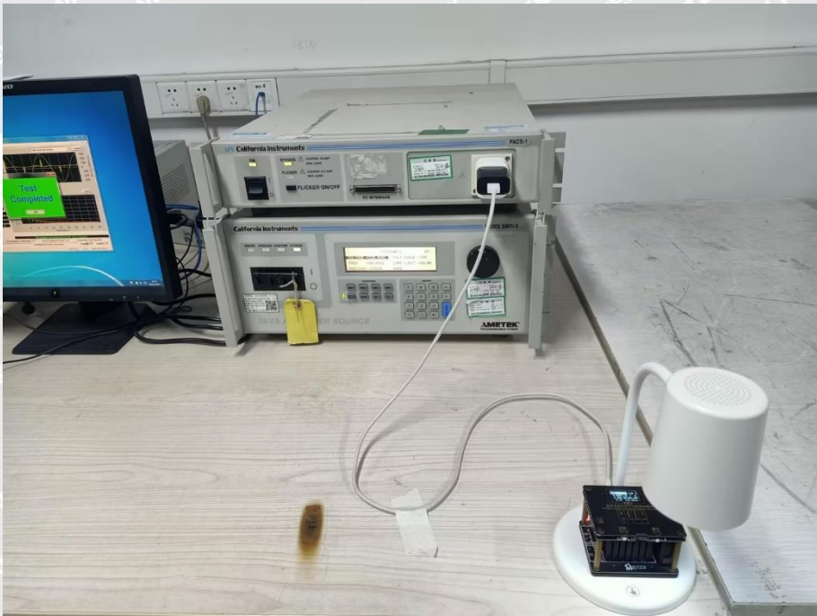
Harmonic/Flicker Test View
