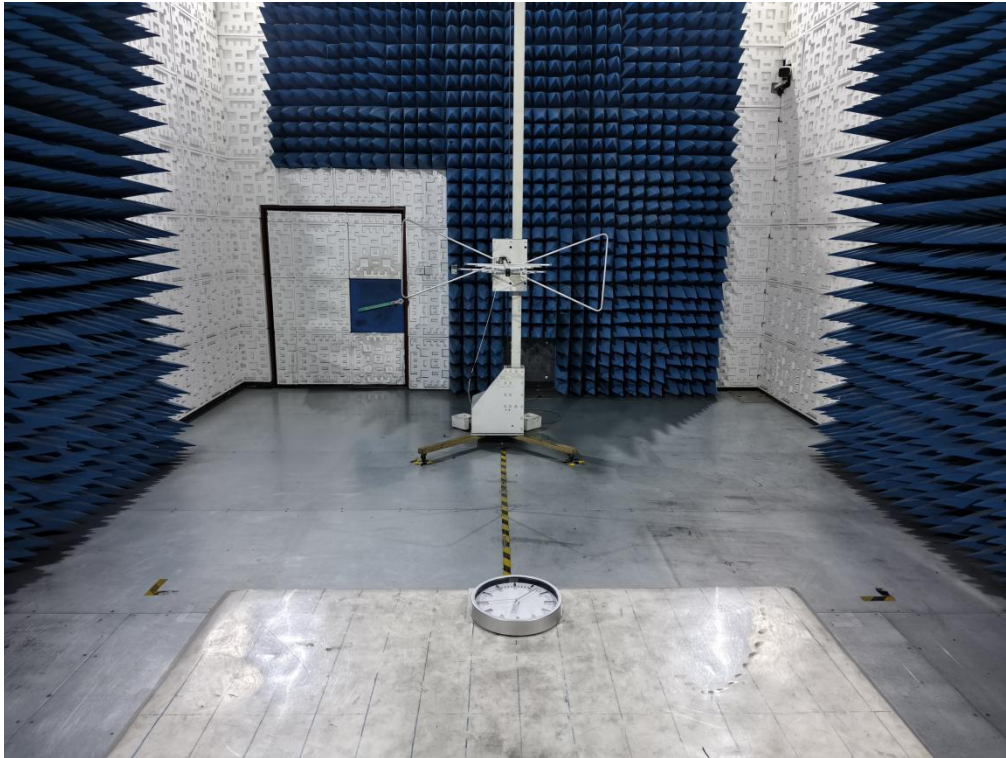
Radiated emissions at frequencies up to 1 GHz
