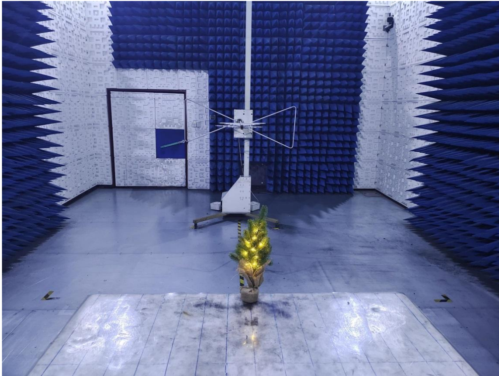
Radiated emissions at frequencies up to 1 GHz
